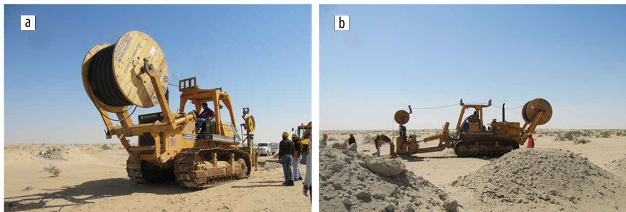
Figure 11. Cable plowing machines deploying continuous cables in shallow trenches as a method of automated placement of DAS seismic cables for surface seismic. (a) A cable spool is carried in front, and (b) a blade at the back splits the ground while the cable is placed at depth by feeding it down a chute located on the back of the blade.
