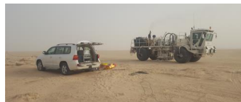
Figure 2. Recording DAS uphole with a mobile unit and vibrator. Single sweep is sufficient since receivers cover entire hole.
