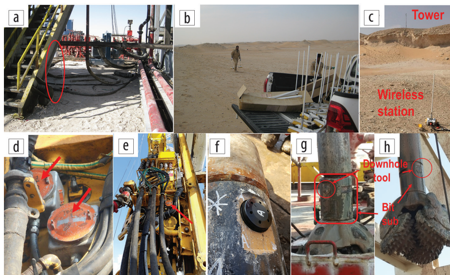
Figure 2. (a) Wireless geophones placed within the rig perimeter. (b) Wireless geophone stations are easy to deploy in the open desert. (c) Transmitting over jebels requires additional radio towers. (d) Top-drive sensors (marked by arrows) are attached to the body of the top drive. The position of the sensors, with respect to the rest of the equipment, can be seen in (e). (f) The downhole tool placed inside the carrier bit sub is shown at the surface. BHA, including the carrier sub and tool, is seen (g) without and (h) with a 28 in roller-cone bit.
