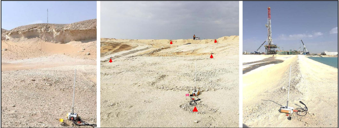
Figure 7—Wireless receiver stations deployed around the rig site recording seismic data while drilling.
