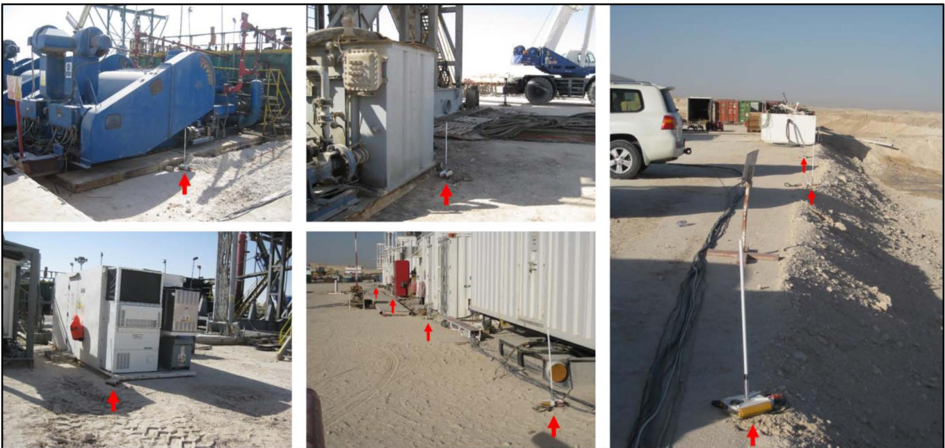
Figure 8—Wireless receiver stations at the rig site.
