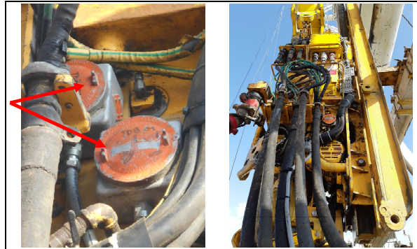
Figure 6. Two orange boxes (a) house top drive sensors attached to the body of the top drive. Their positioning with respect to the rest of the equipment can be seen on (b).
