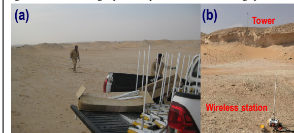
Figure 4. Placement of wireless geophone stations (a) and transmitting over jebels with additional radio tower (b).
