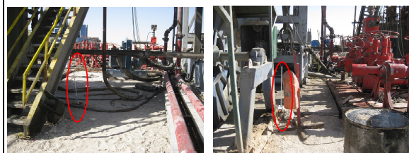
Figure 3. Wireless geophones placed within the rig perimeter.
