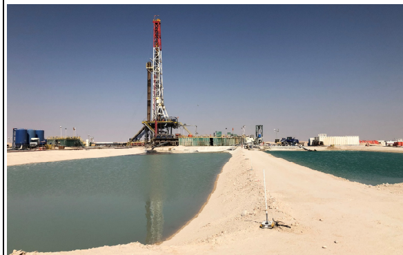
Figure 2. DrillCAM field trial at an onshore rig. Line of wireless geophones with antennas is seen going towards the rig.
