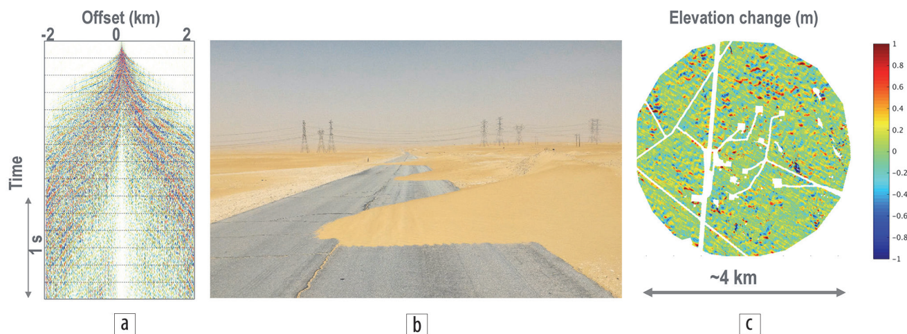
Figure 1. The main challenges faced by time-lapse seismic in a desert environment include (a) low S/N levels on recorded data and (b) constantly shifting sand dunes resulting in (c) changes in topography shown over a two-year period.
