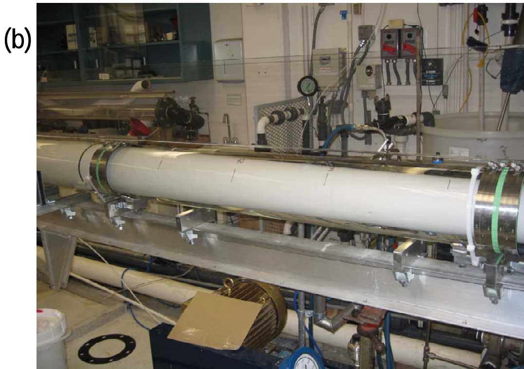
Figure 4: (a) Sketch of the flowloop setup with the model of sand-screened completion in horizontal well. (b) Photograph of the actual flowloop setup at Shell's Bellaire Technology Center with a glass outer pipe (no perforations).
