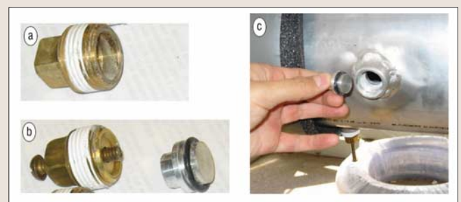
Figure 11. Two types of perforation plugs used in the experiment: (a) smaller plug that leaves part of the perforation tunnel open (height of \sim 2 cm); (b) large (two-component) plug that completely fills the perforation tunnel; (c) picture showing installation of the bottom component of the large plug.
