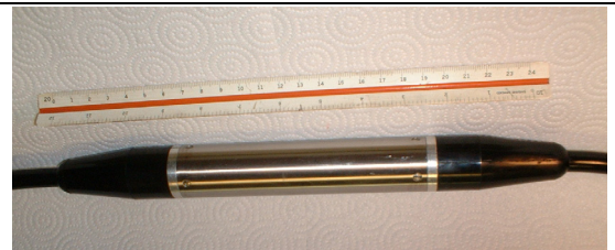
Figure 4: 4C sensor from VSP array for shallow boreholes (courtesy of Don Fussell, VCable LLC).
