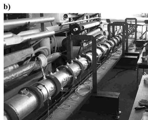
Figure 2. (a) Sketch and (b) photograph of the full-scale laboratory model of a completed horizontal well.
